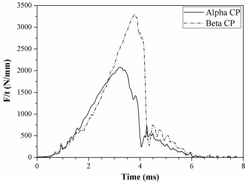
Characteristic IFWI fractograms in the form of thickness-related force ( $F/t$ ) vs. time for the CP homocomposites.
