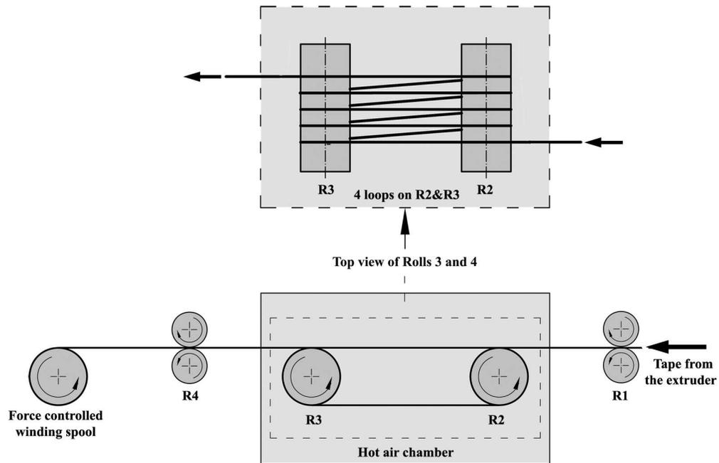
Schematic sketch of the hot stretching unit. Note: the speed of the rollers R1, R2 and R3 was the same, while that of R4 varied in order to set the required draw ratio (DR).
