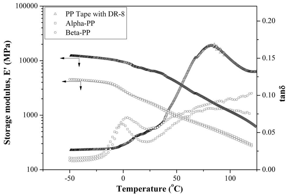
Storage modulus ( $E'$ ) and  $\tan\delta$  vs. temperature curves for the alpha- and beta-PP, and PP tape with DR-8.
