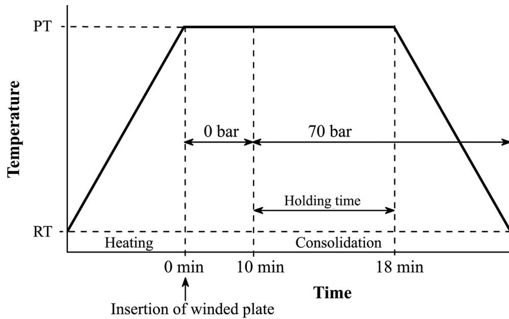
Processing cycle for hot pressing of the PP homocomposites.
