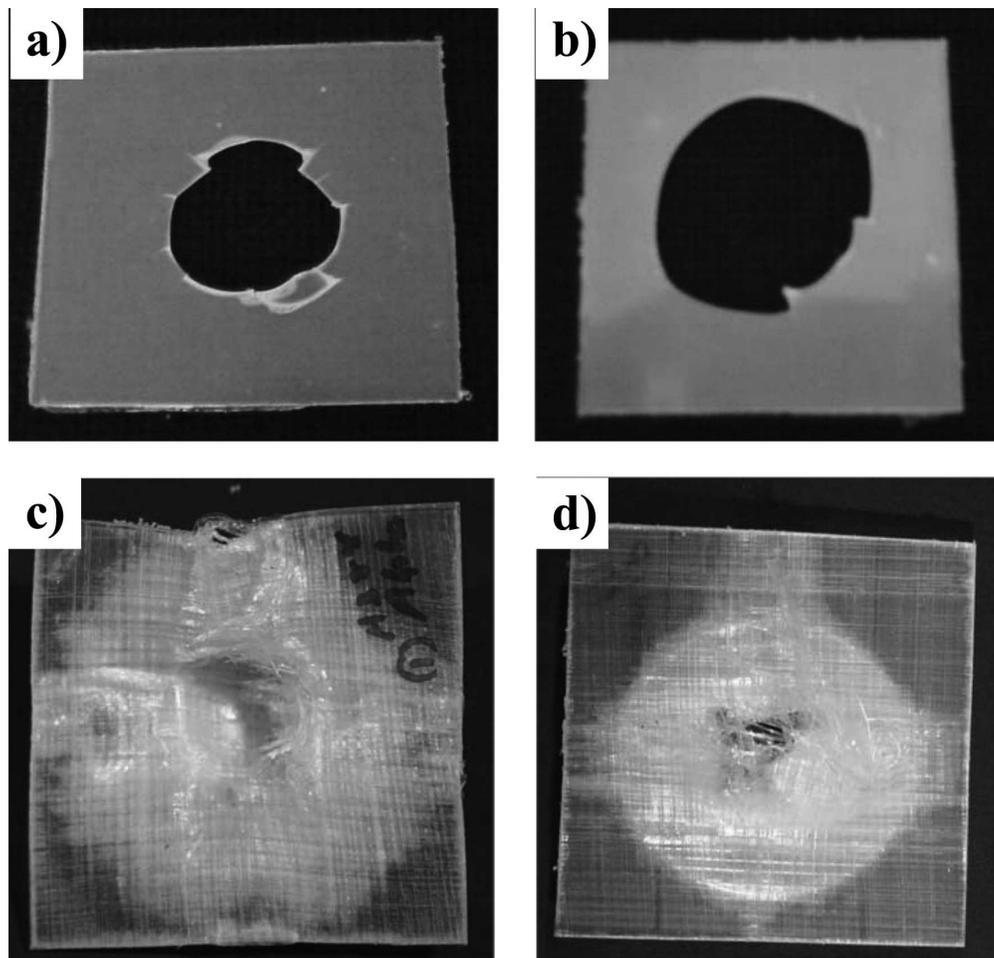
Top views of the failed IFWI specimens of alpha- (a) and beta-PP (b) matrices, and alpha CP (c) and beta CP homocomposites (d). Note: the dimension of the impacted specimens is 60x60 mm<sup>2</sup>. 150x144mm (300 x 300 DPI)
