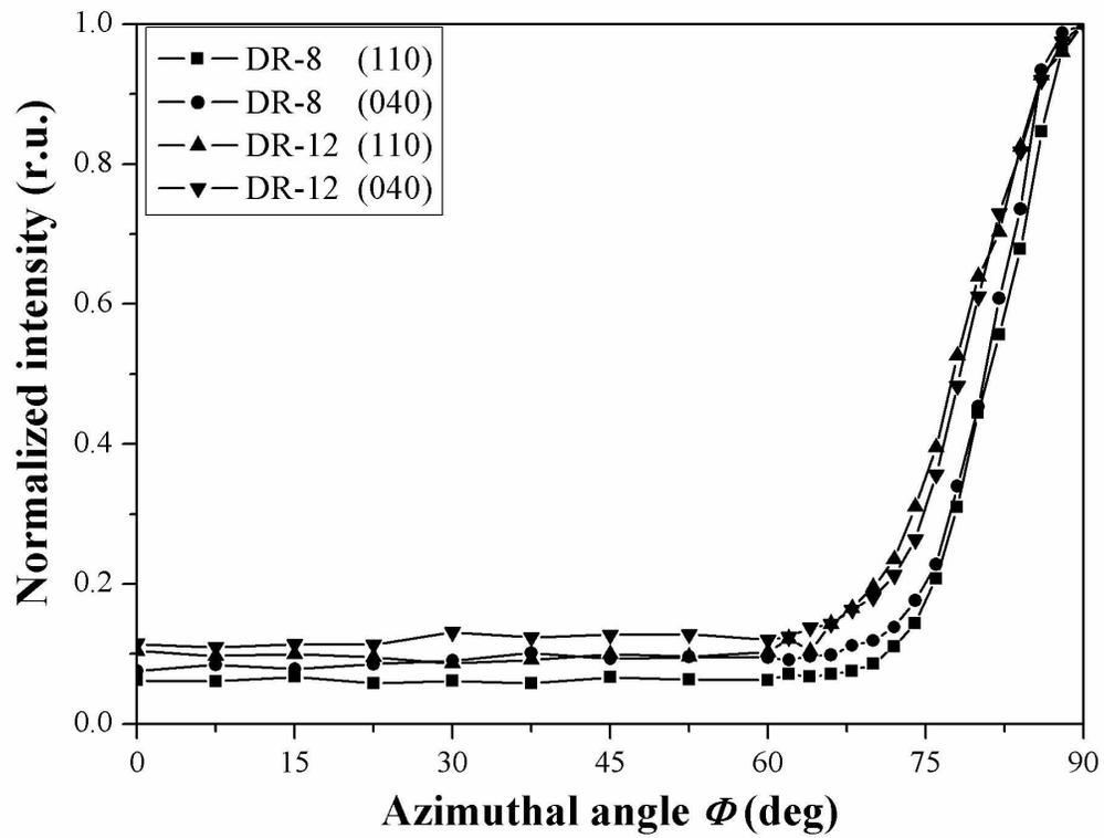
Azimuthal scans for the PP tapes of DR-8 and DR-12 over the 100 and 040 reflexes. Note:  $\Phi$  is the angle between the chain axis of PP and the stretching direction.
