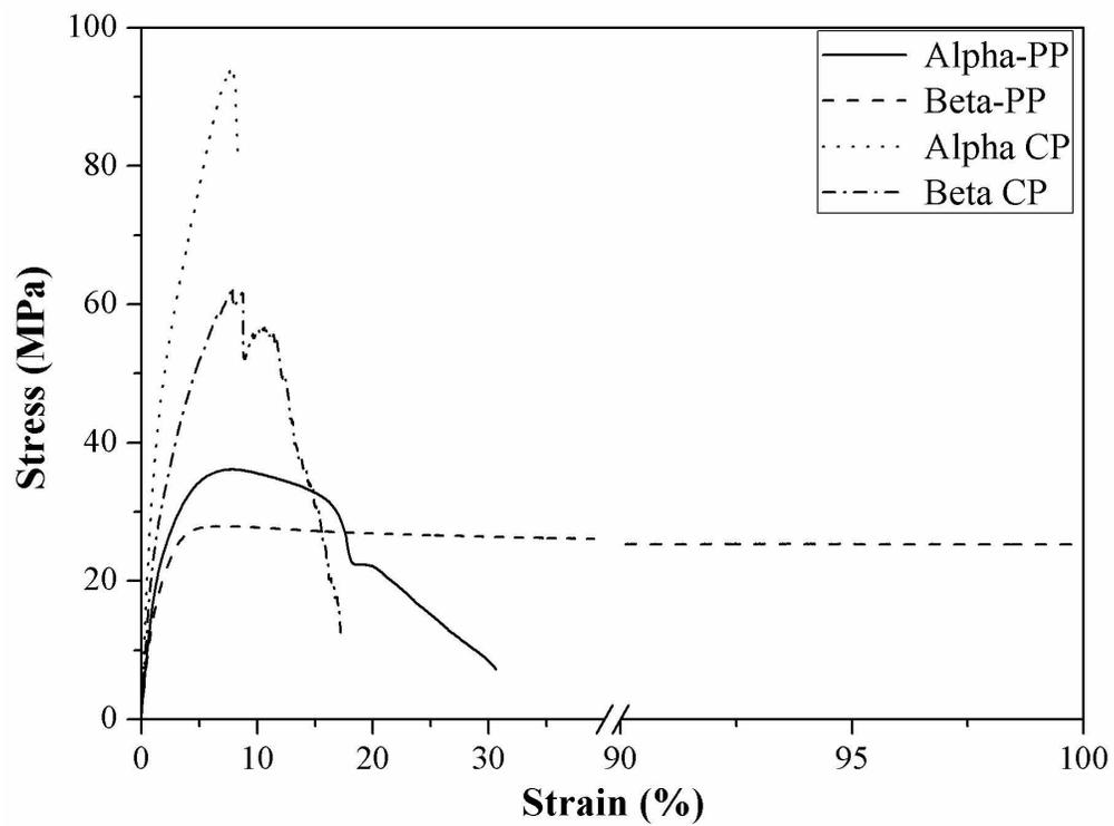
Stress-strain curves for the PP matrices and corresponding CP homocomposites.
