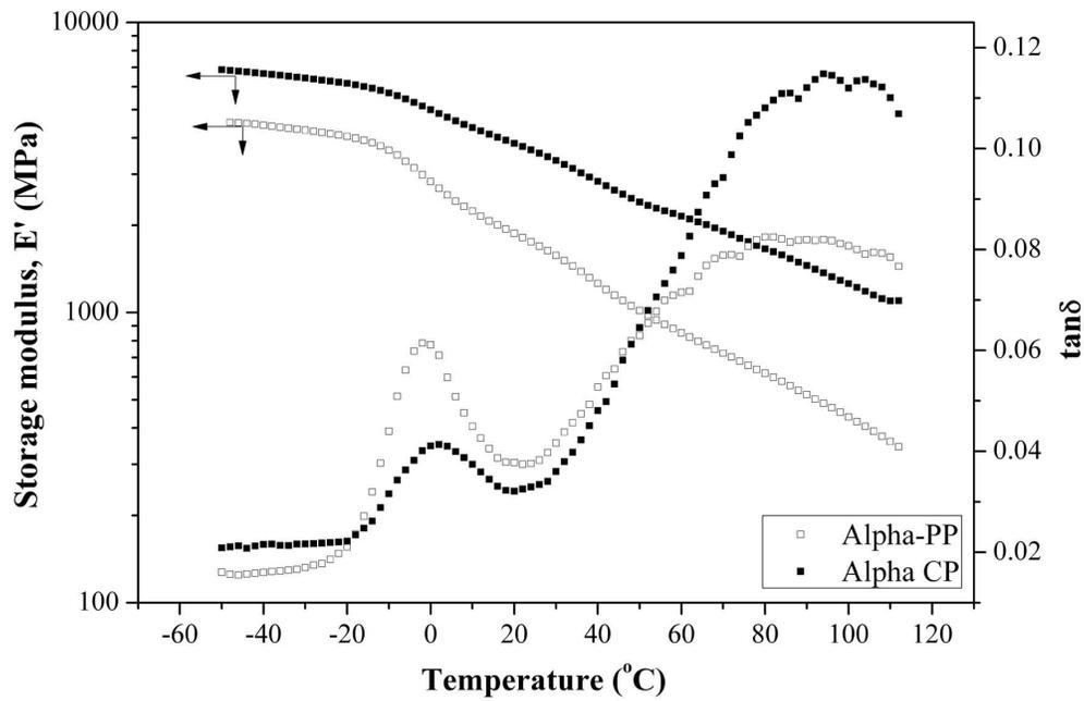
Storage modulus ( $E'$ ) and  $\tan\delta$  vs. temperature curves for alpha-PP and its homocomposite (alpha CP).
