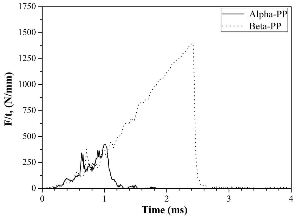
Characteristic IFWI fractograms in the form of thickness-related force ( $F/t$ ) vs. time for alpha- and beta-PP.
