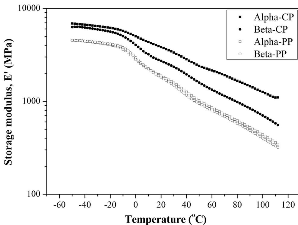
Storage modulus ( $E'$ ) vs. temperature curves for the PP matrices and corresponding homocomposites.
